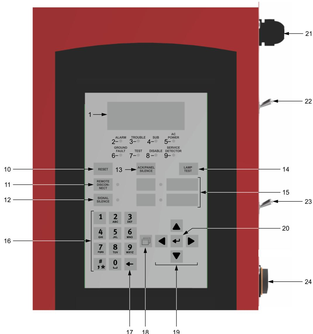
**Figure 2.** Display and LEDs of the FACP.
